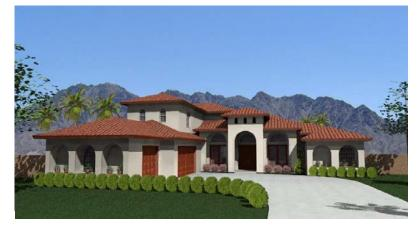
A **hip roof**, or **hipped roof**, is a type of roof where all sides slope downwards to the walls, usually with a fairly gentle slope. Thus it is a house with no gable or other vertical sides to the roof. A square hip roof is shaped like a pyramid.
